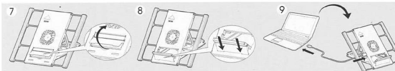
7. Lift the Shelf Support Bracket upwards as shown.
