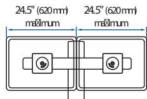
This range accommodates most displays with screens up to 24" as well as some displays with screens as large as 26".
